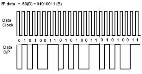
Verify data O/P waveforms for other BCD inputs.
