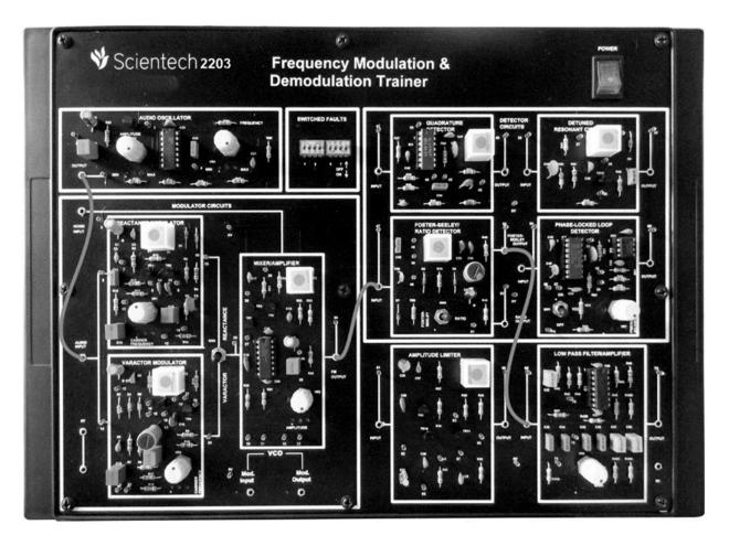
Figure 5 Connections for FM Demodulation using Foster-Seelay Detector
