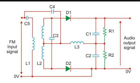
Figure 3 Foster – Seelay Detector
