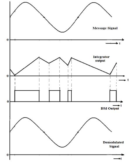
Waveforms of Delta Modulation & Demodulation
