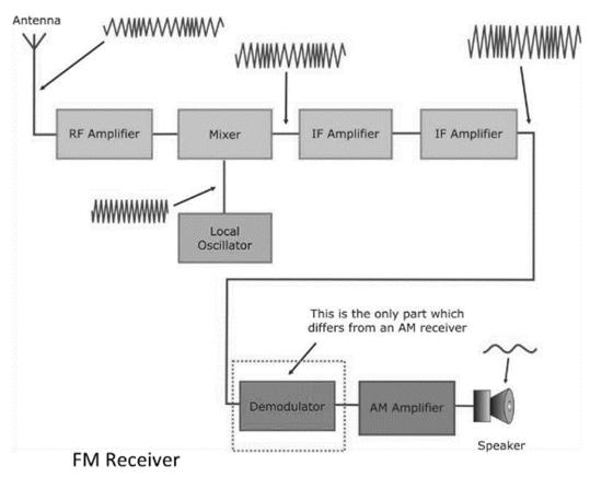
A FM receiver is very similar to an AM receiver. The most significant change is that the demodulator must now extract the information signal from a frequency rather than amplitude modulated wave. The basic requirement of any FM demodulator is therefore to convert frequency changes into changes in voltage, with the minimum amount of distortion. To achieve this, it should ideally have a linear voltage/frequency characteristic. A 'demodulator' can also be called a 'discriminator' or a 'detector'.
