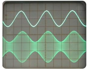
Since Scientech 2201 TX output select switch is in the ANT position, the AM signal at the output is fed to the transmitter's antenna. Prove this by touching Scientech 2201's antenna, and nothing that the loading caused by your hand reduces the amplitude of the AM waveform at the output.
