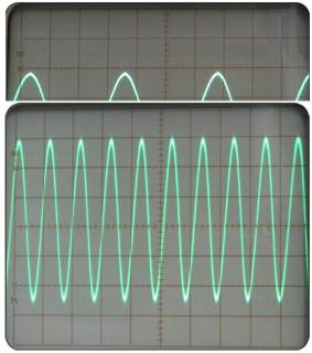
Step 4 1 MHz Crystal Oscillator Block generates a sine wave of 1 MHz frequency and 120mV pp amplitude approx, which is used as a carrier input to Balance Modulator and Band Pass Filter Circuit 1. Observe the carrier waveform at output test point on Oscilloscope. [CH1(Y) – 10mV; Time base – 1 uS]
