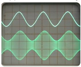
Step 6 To determine the depth of modulation, measure the maximum amplitude  $(V_{\text{max}})$  and the minimum amplitude  $(V_{\text{min}})$  of the AM waveform, and use the following formula:
