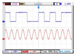
CH1: Input Data Clock (TP1), CH2: Input Data(TP2)
