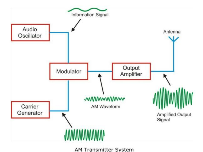
Amplitude Modulation is the process of changing the amplitude of a relatively high frequency carrier signal in proportion with the instantaneous value of the modulating signal. The general equation of Amplitude Modulated signal is given by
