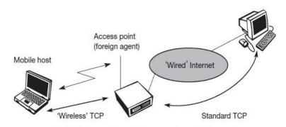
Fig. I-TCP segments a TCP connection into two parts
