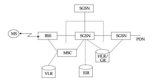
Figure 2.2.1 GPRS Architecture Reference Model
