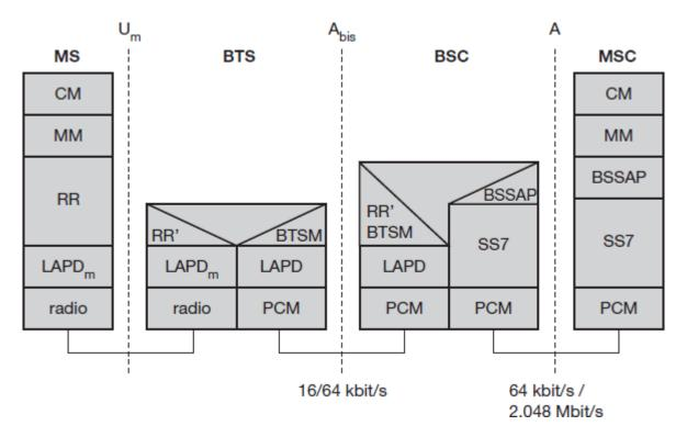
Figure 2.1.3 Protocol architecture for Signalling
